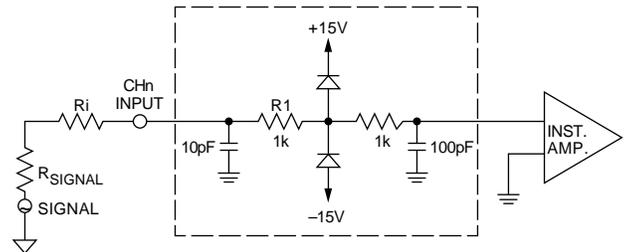
Figure 3. Multiplexer Equivalent Circuit
