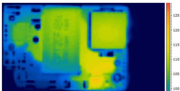
SB24S15-1 Thermal Image 1A output, 85C Ambient, Natural Convection V_{in} = 24V , (airflow from pin 3 to pin 1, T_{max} = 105^{\circ}C )
